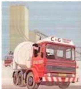
Powered by the Leyland fixed head 0.500 engine of 8.2 litres, these were all fitted at Stamford with Allison automatic transmissions, which gave safer driver control, particularly reversing on delivery sites. Our livery changed from maroon cab and light battleship grey mixer to the current white and red scheme.
